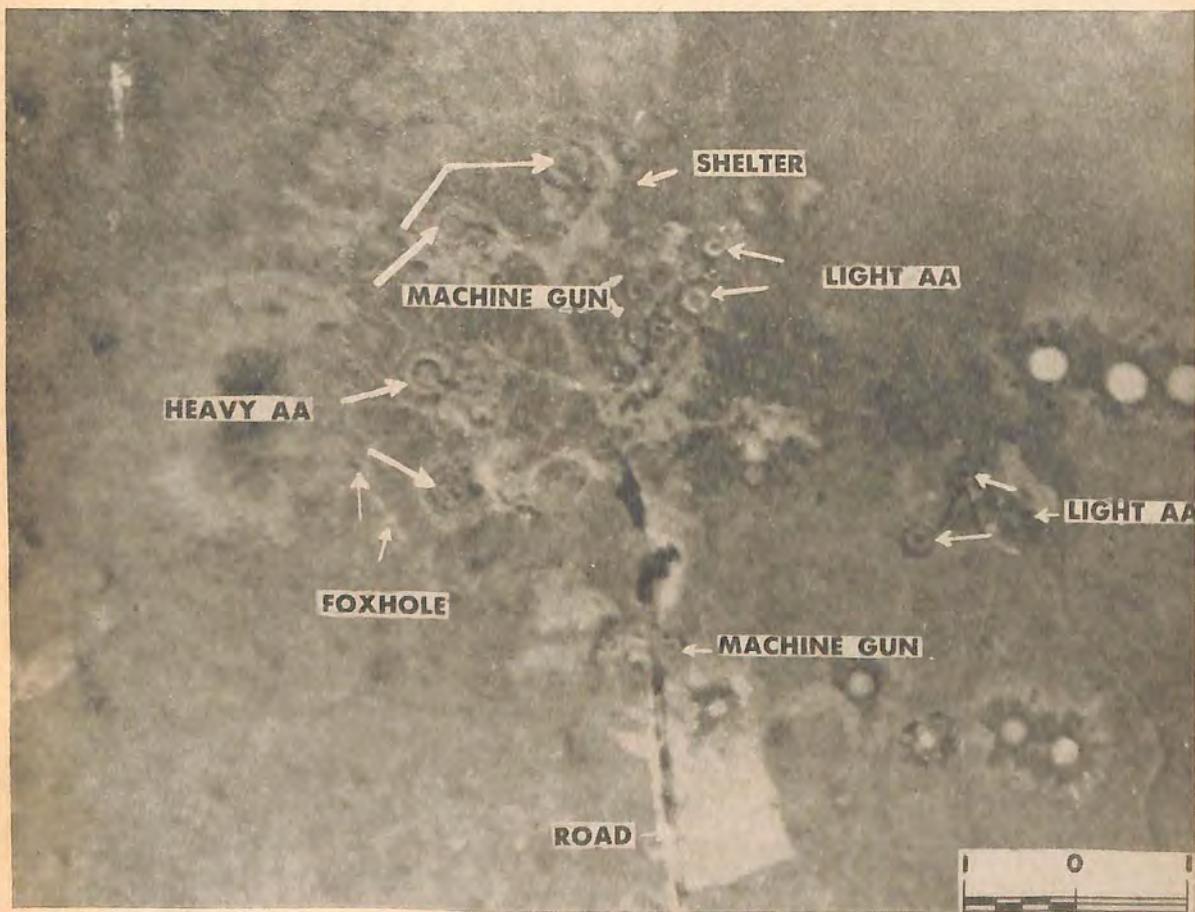
Figure 89. Four Gun Heavy Anti-aircraft Battery (Emplacements Empty). Emplacements are built of earth over which grass has grown. Pattern is a shallow arc with fire control installations in center. A three-gun light anti-aircraft are also present. The large emplacements could house 75-mm or 105-mm guns. The small emplacements are probably for heavy machine gun or 13-mm anti-aircraft.
